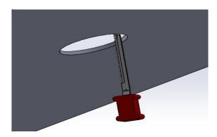
3. Pull the electric cable through the hole .connect the main supply to the luminaire & secure connections with wire connectors and tuck them inside the fixture junction box .
