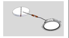
4. Press the mounting clamp & Insert the luminaire into the ceiling hole & secure the luminaire using the provided clamp . Insure it is flush with ceiling and stable .
